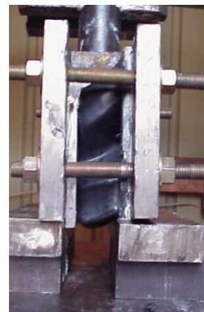
Figure 6: Tension pad at 40,000-pound load
