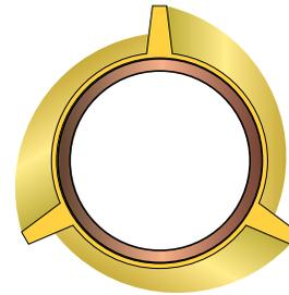
Mark's UreGuard VIV breaks up currents that cause vortex-induced vibrations.
