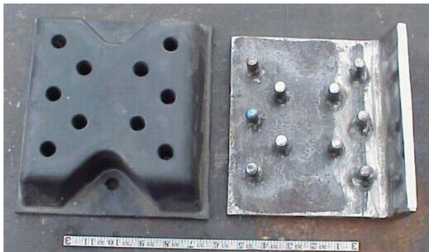
Figure 1: A photograph of a submitted tension pad with fabricated load application plate.
